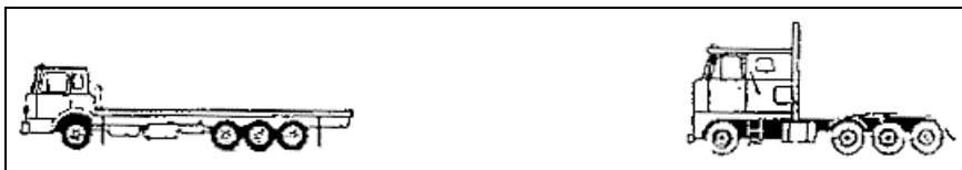
FHWA Class 6/7, Single unit trucks with more than two axles
